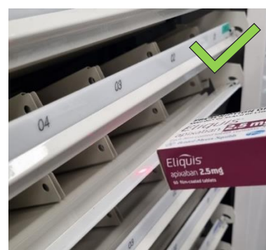
Figure 3: An example of correct loading, where the package is being loaded flat side down.
