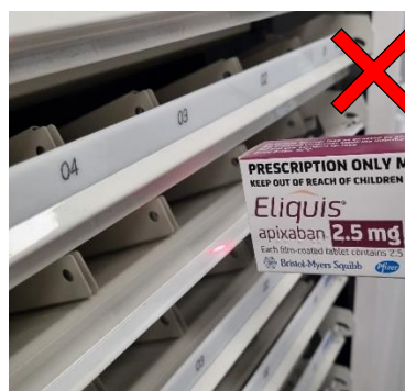
Figure 19- An example of incorrect loading, where the package is being loaded on a tall edge.
