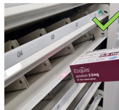
Figure 20- An example of correct loading, where the package is being loaded flat side down.
